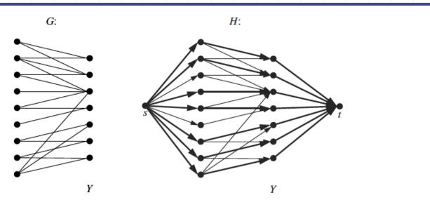
**Figure 16.11:** (a) A bipartite graph G. (b) Flow network H derived from G and a maximum flow in H; thick edges have unit flow and other edges have zero flow.
